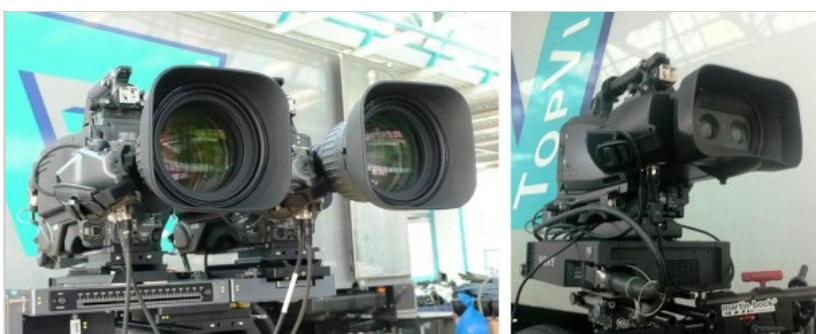
Sony HDC-1500 on Elemet Technica Side-by-Side rig and Sony PMW-TD300
